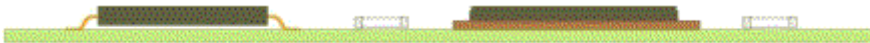
Fig 1a Tested, burned-in packaged components are aligned on an insulating base and bonded in exact positions.
