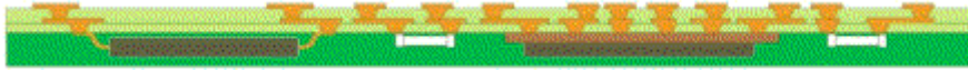
Fig. 1f A second conductor plating fills the vias and provides added interconnectivity. Further layers can be deposited if needed by repeating 1e and 1f.
