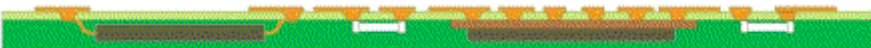
Fig. 1d A conducting circuit layer is plated on the top surface of the base in a build-up
