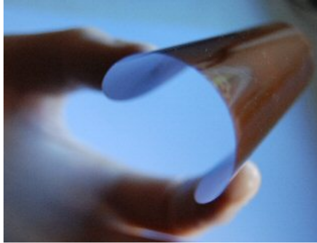
Figure 3. Polyimide substrate flexibility.
