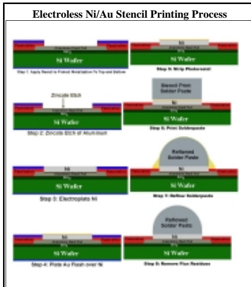
Figure 4: Electroless Ni/Au UBM followed by Stencil Printing Process
